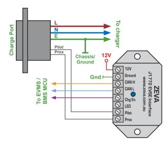
The LED terminal will mirror the behaviour of the LED on the device, optionally used for powering a remote LED in a more visible location. The output has a 5mA current limit (no series resistor required).
